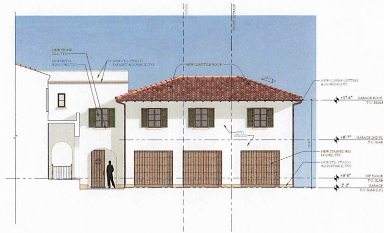
4 PROPOSED SOUTH GARAGE, VIEW FROM PORTE COCHERE 3/16"=1'-0"
