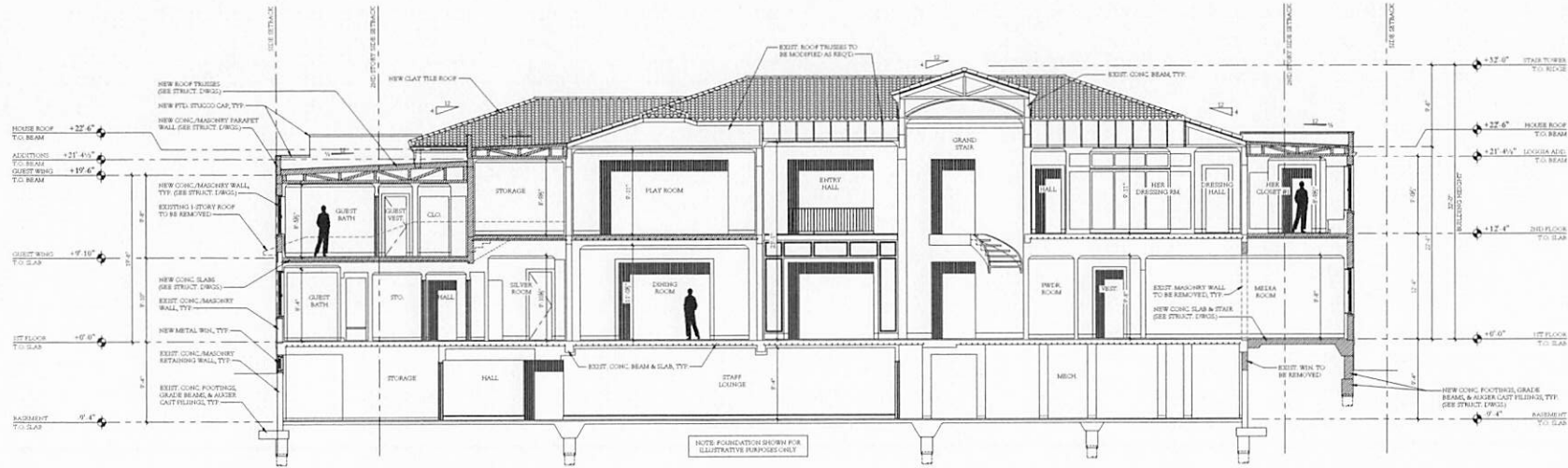
1 BUILDING SECTION AT ENTRY HALL, LOOKING EAST 3/16"=1'-0"
