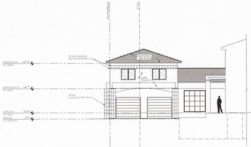
1 EXISTING NORTH GARAGE, VIEW FROM PORTE COCHERE 3/16"=1'-0"
