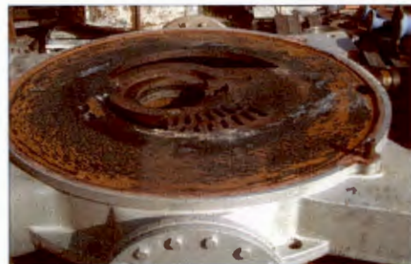
Erosion-corrosion damage on port plate
