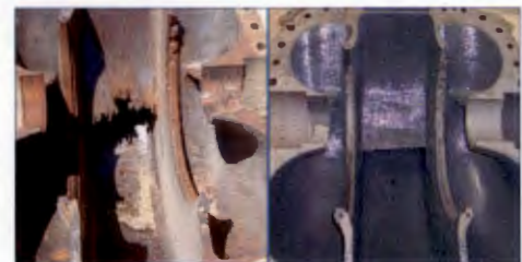
Typical effects of erosion-corrosion on a centrifugal pump cutwater
