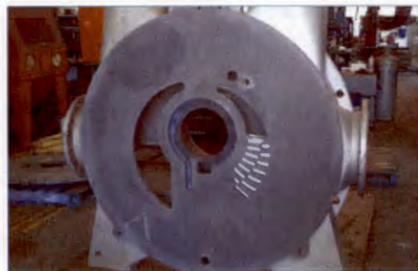
Port plate repaired with Belzona 1111
