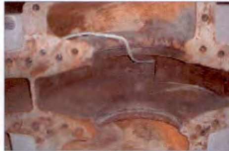
Corroded and cavitated pump
