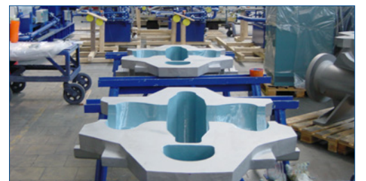
Belzona 1341 (Supermetalgilde) used by an OEM
