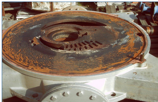
Erosion-corrosion damage on port plate
