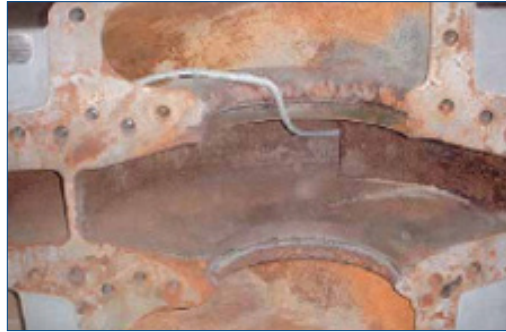
Corroded and cavitated pump
