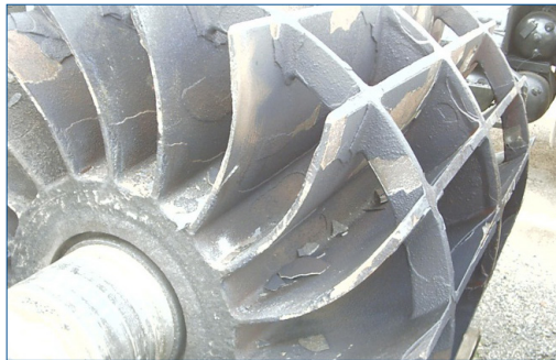
Damaged rotor before rebuilding
